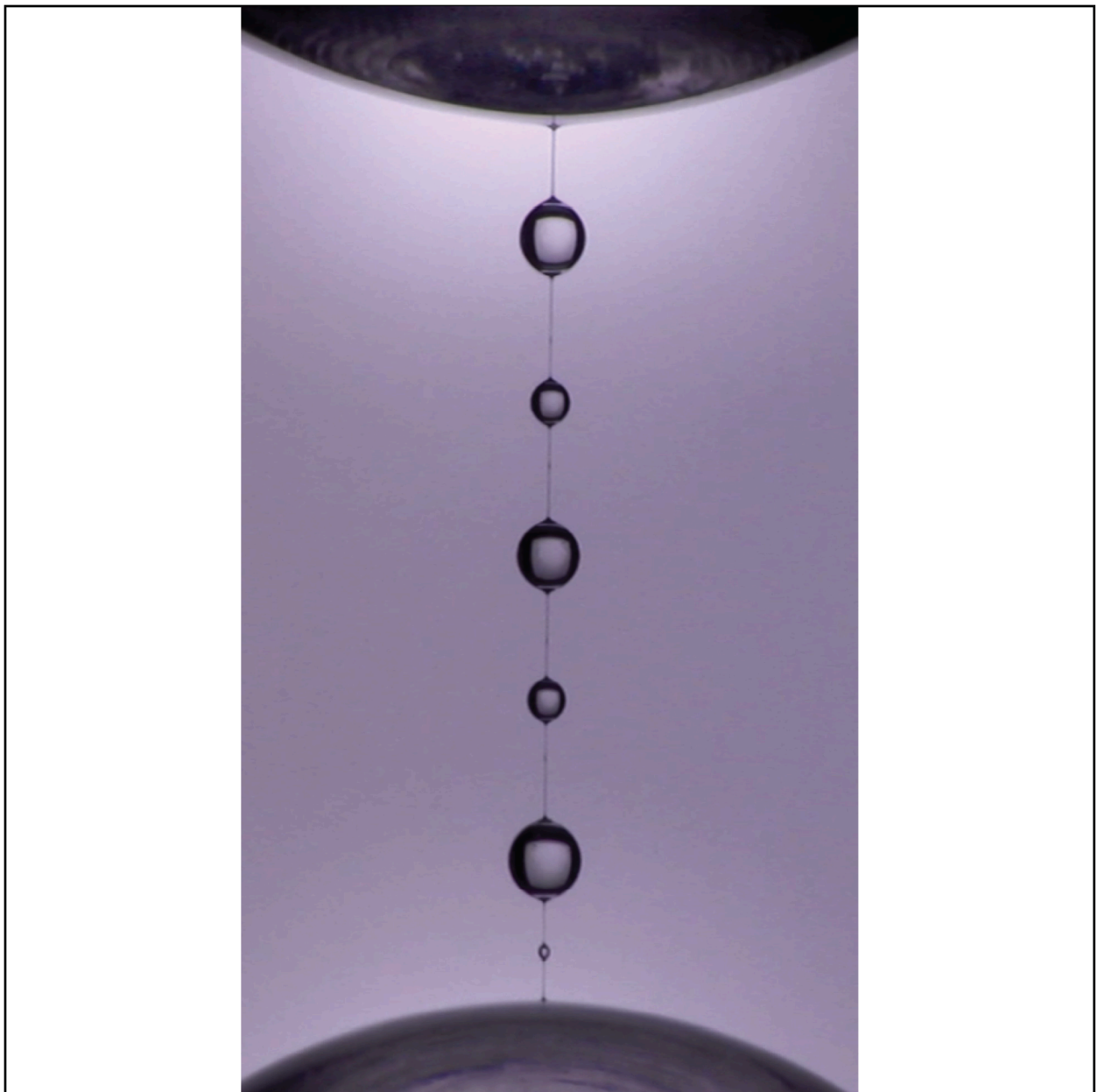
A "beads-on-a-string" structure forming in a thinning saliva bridge, which is a viscoelastic fluid. Here, polymers in saliva (mucins) resist the capillary-
